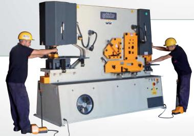
Two operators can work simultaneously on double pistons models (HKM 55-65-85-115-175)
